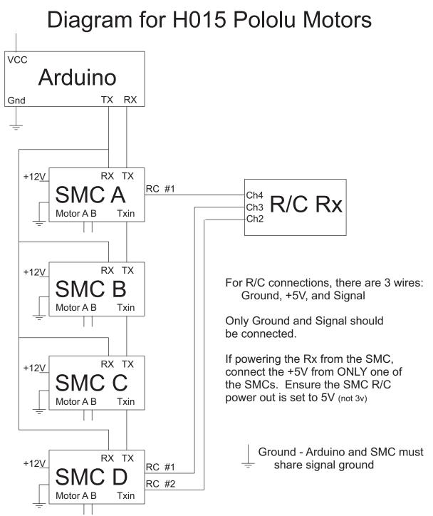
Optionally TX of "D" could go to TXin of "A" and skip TX of B & C completely +12V should be appropriate motor voltage, could be +24V or other values
